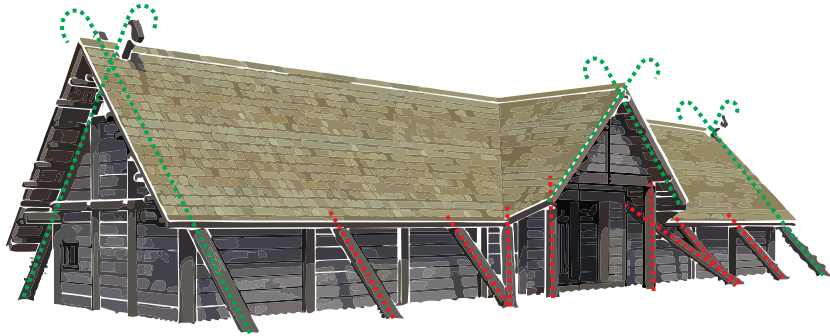
The dotted lines are your roof supports
